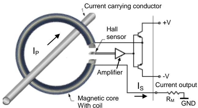
The magnetic flux created by the primary current  $I_p$  is balanced by a complementary flux produced by driving a current through the secondary windings. A hall sensor and associated electronic circuit are used to generate the secondary (compensating) current that is an exact representation of the primary current.
